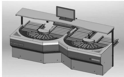
The operators will stand in front of the screen, with retrieved stock delivered on one conveyor. The operator will consolidate the orders and place them on the other conveyor, to be passed on to the packing team before they are dispatched.
